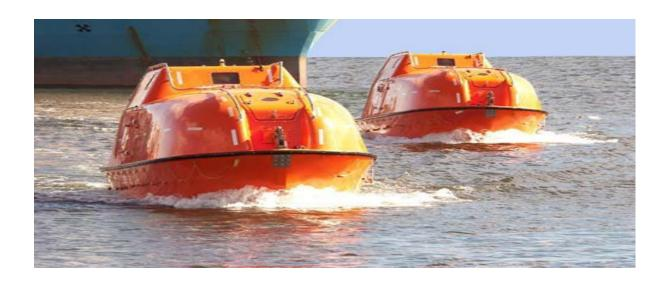
4 off SC102 83 Person totally enclosed tanker version lifeboats (EU Spec), 98 Kgs per person (533mm seat) – 4 off Acebi Electric Winches for Cantilever-davit Type supplied / please note: no davits supplied
